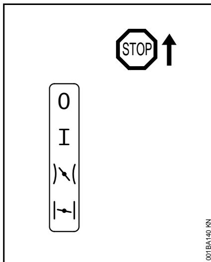
**Stop 0** – engine off – the ignition is switched off
