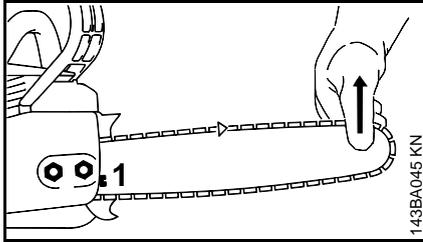
Retensioning during cutting work:
