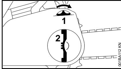
Retensioning during cutting work:
